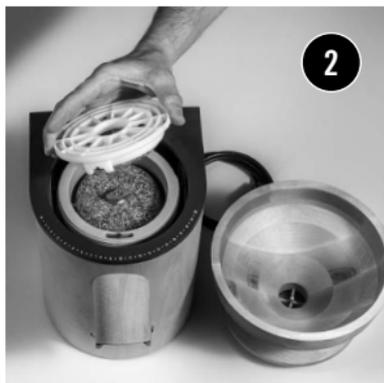
If a hard film has built up on the stones please see page 17 where we show how such a film can be removed. Now the stator can be put back into place. Then you can remove grain residue from the milling chamber and clean the two stones using a soft brush or a wooden spatula. Be careful not to lose the two small springs that support the upper stones!
